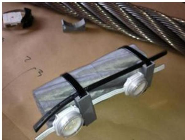
Above, one of the Bay Lights modules, with a sample of the cable it will be attached to. 3d Printing has been used in the prototyping.
